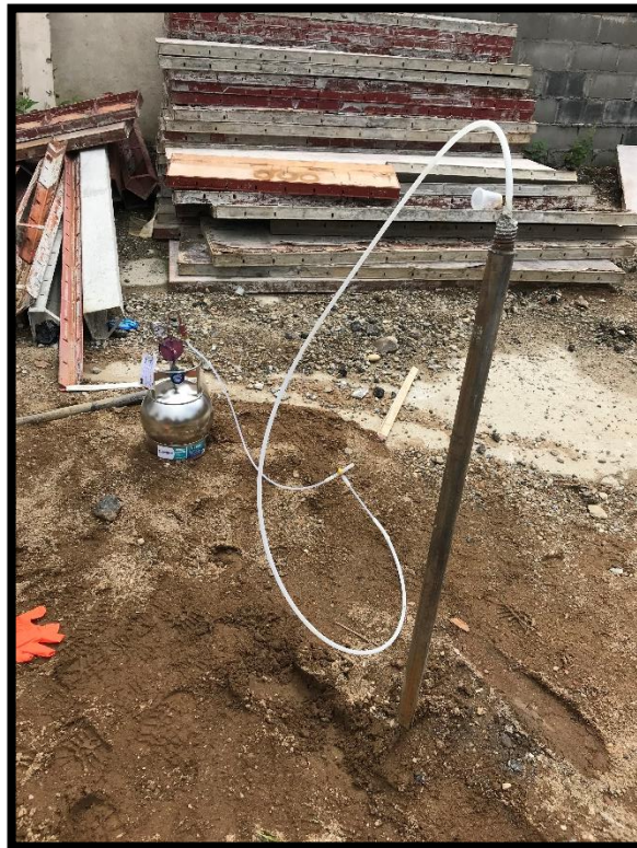
SSSG(Subslab Soil Gas) sampling at SB-4
