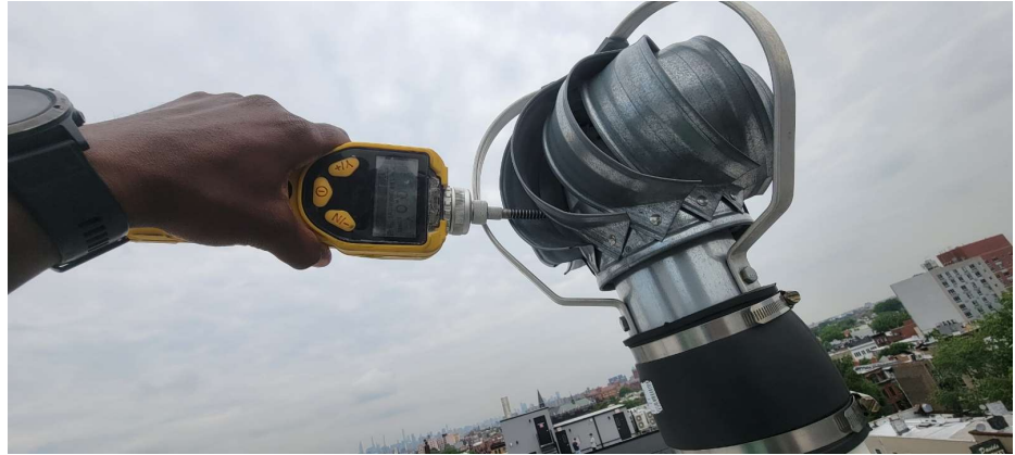
Organic vapors measurements at the SSD system riser
