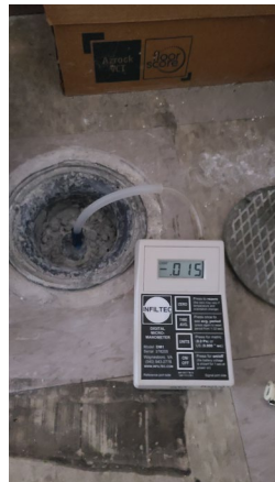
3. Typical digital manometer reading, SSMP VM-05
