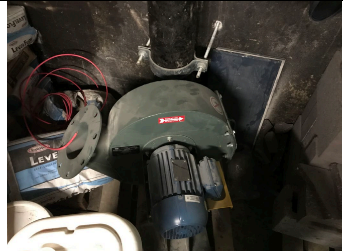
Photo 8: Spare SSDS fan stored in cellar of school building.
