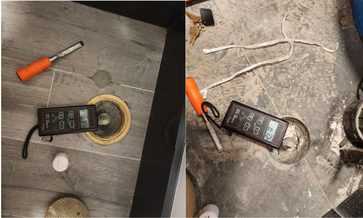
Photo 7 and 8 – View of manometer readings from the two monitoring points on Site for the SSDS.
